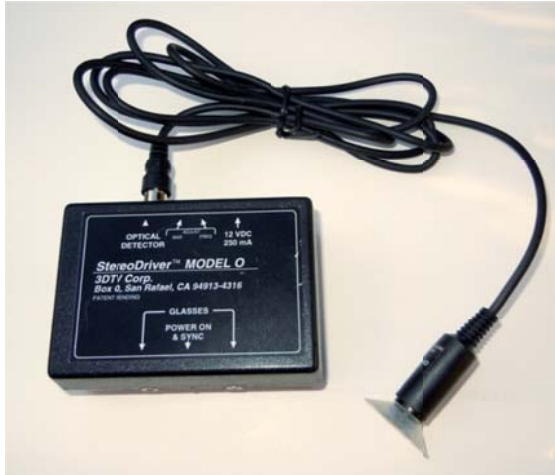
From the archives of electronic stereoscopy—the 3DTV Corp Model O wired shutter glasses system from 1994 picked up sync from the TV screen with a photodiode in a suction cup.
