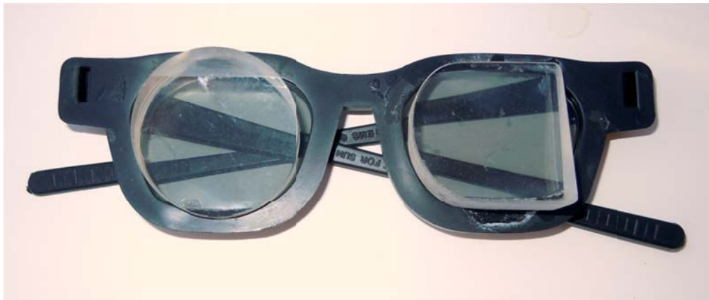
Wedge prism glasses I made in 1983 for viewing top/bottom stereo TV, or for chromostereopsis (i.e., depth from color alone—a concept later made popular by the ChromaTek glasses developed by Rick Steenblik and marketed by APO). Chromostereopsis was first investigated by the famous German physicist Hermann Von Helmholtz and described in his classic book on Physiological Optics.
